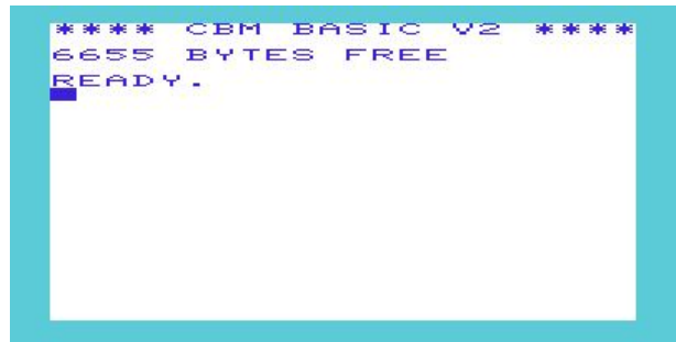
VIC-20: 3K expanded BASIC: $0401, Screen:$1E00, Color:$9600 (can be disabled by typing: POKE642,16:POKE644,30:SYS64818)
